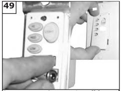
Remove cover by snapping off from top or bottom. Install 12V battery into wall remote. Duracell MN21/Eveready A23/GP 23A all 12V
